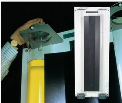
Subsonic Wind Tunnel - C2 Measuring lift and drag forces
