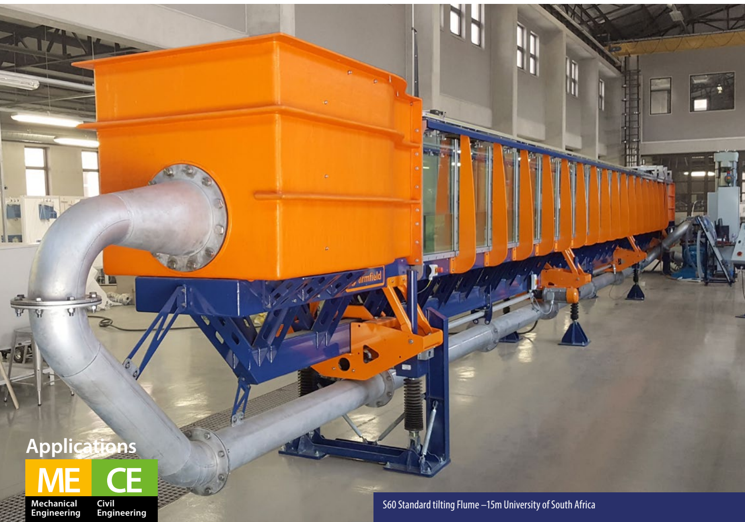
S60 Standard tilting Flume –15m University of South Africa S6-MkII Standard tilting Flume –15m University of South Africa
