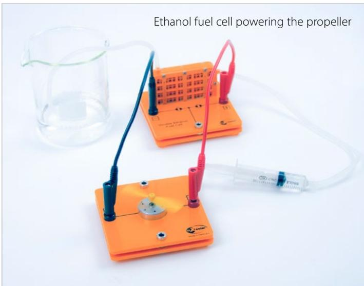
Ethanol fuel cell powering the propeller
