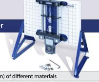
Tensile tests (to destruction) of different materials Finding the tensile strength of a material Material behaviour in the elastic and plastic region Creating a force and extension chart
