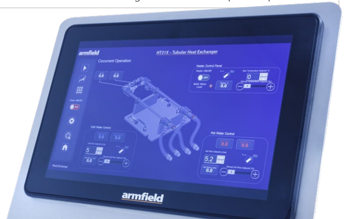
Software screen for HT31X, PID control of temperature and flow
