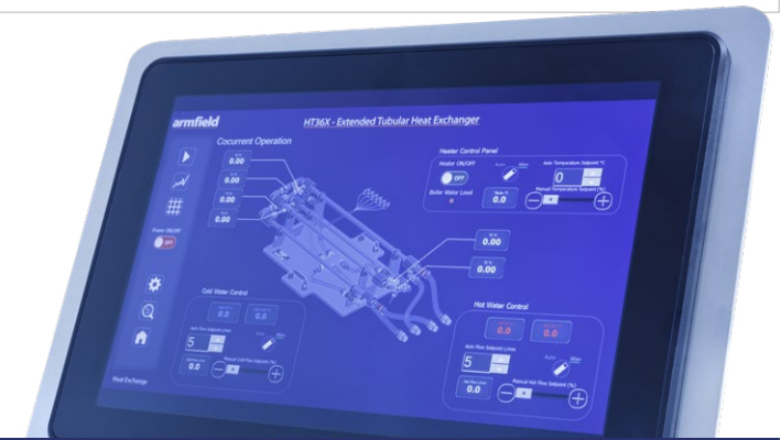
Software screen for HT36X, PID control of temperature and flow
