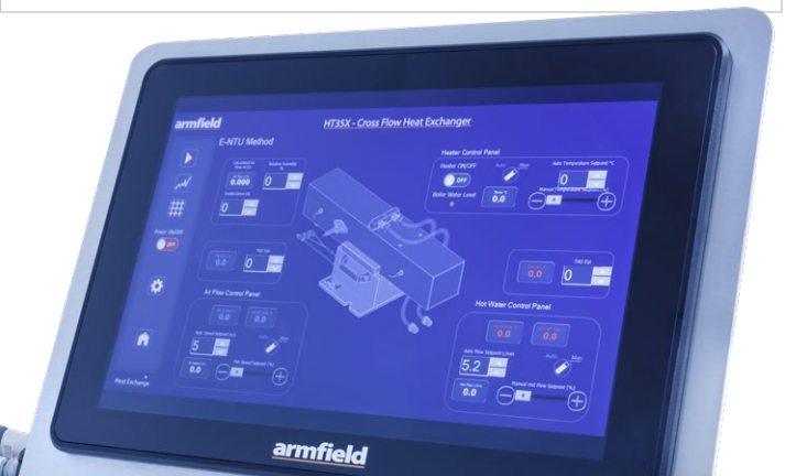
Software screen for HT35X, PID control of temperature and flow
