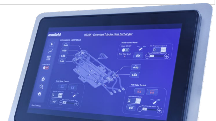
Software screen for HT36X, PID control of temperature and flow
