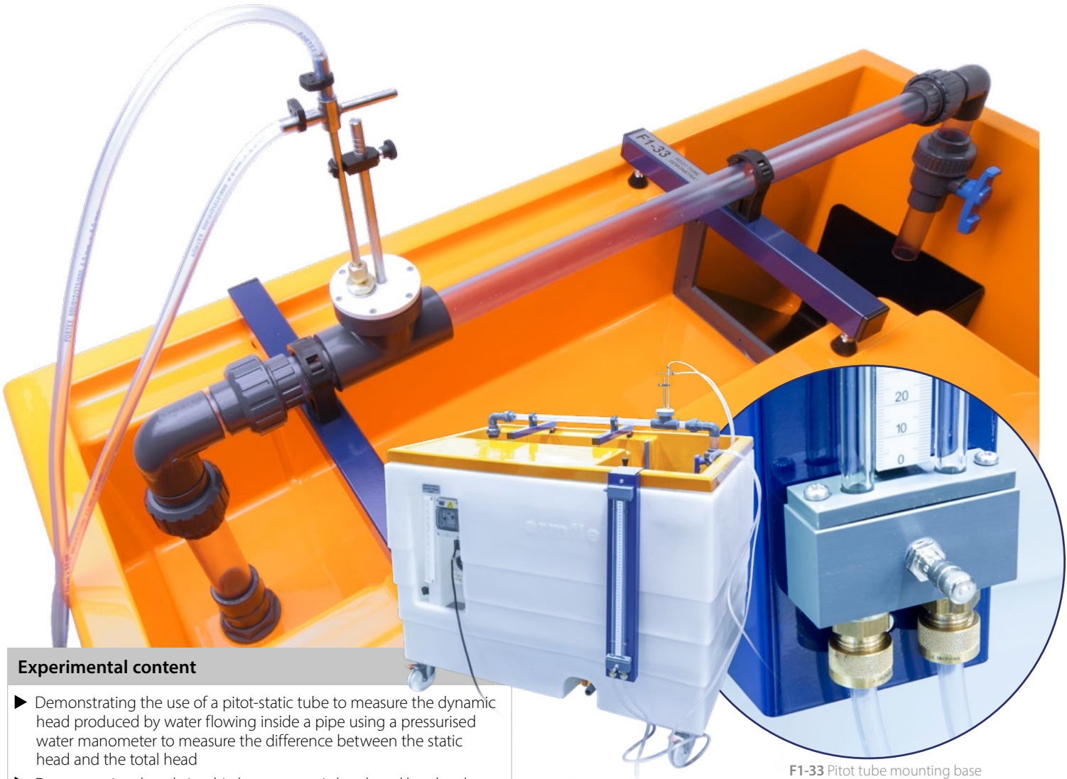
F1-33 Pitot tube mounting base
