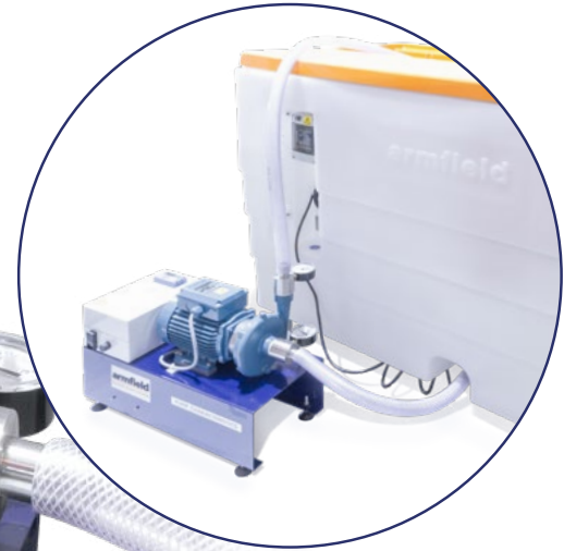
F1-27 Centrifugal pump attached to F1-10 bench
