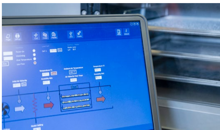
Control screen showing the mimic diagram, the UOP8MKIIe can be controlled remotely
