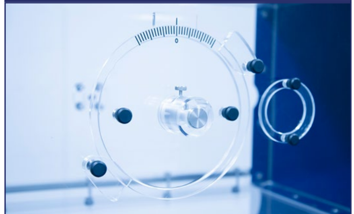
Instrumentation mounting points in the side wall and roof, with further model access via the floor
