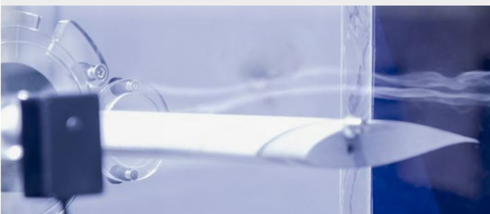
The probe smoke generator allows for easy visualisation of the air flow
