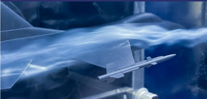
The probe smoke generator allows for easy visualisation of the air flow
