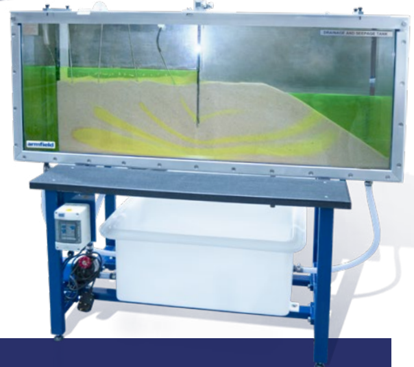
S1: Seepage under a sheet pile wall
