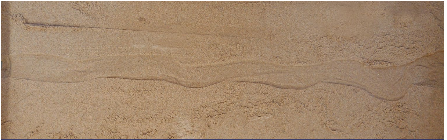
Initial straight channel developing meandering behaviour after a time period
