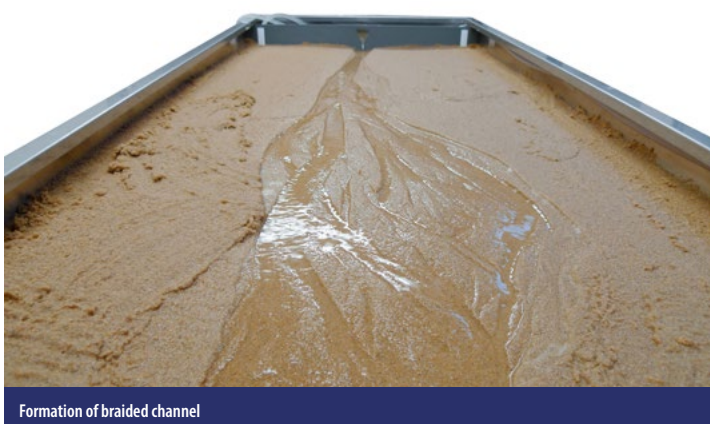
Initial straight channel developing meandering behaviour after a time period
