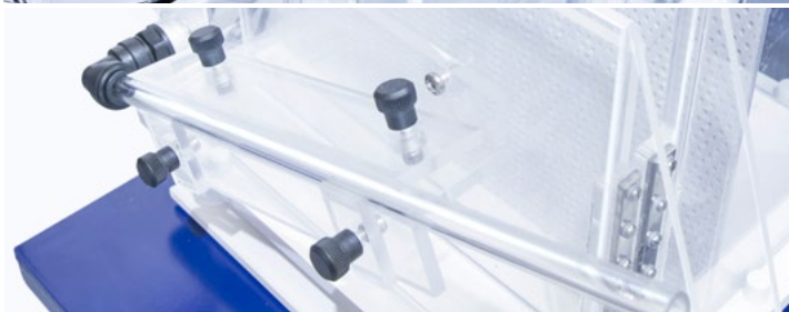
Inclined manometer for measuring of the height over the notch weir
