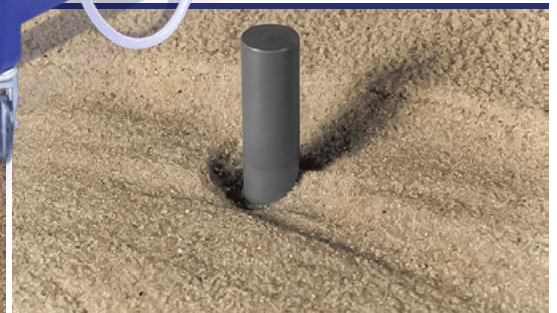
Example of scour in open channel flow around a circular bridge pier
