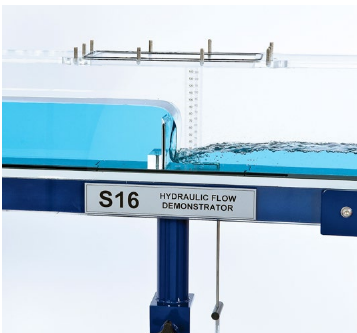
Flow over a sharp crested weir with the nappe (unventilated) clinging to the downstream face
