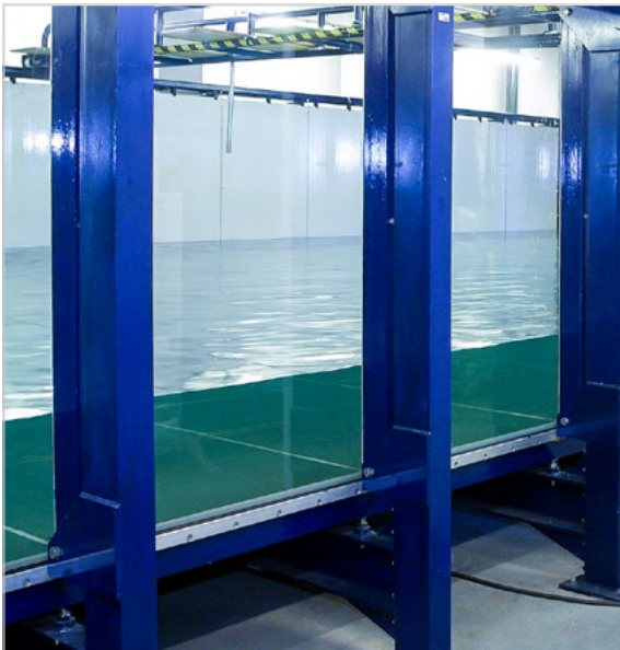
The University of Exeter flume in use for a sediment transport experiment
