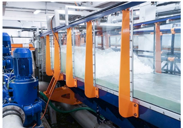
S Series Static Flume: Wind over wave with counter current flow
