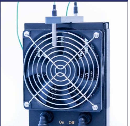
Cross flow heat exchanger fan and sensors
