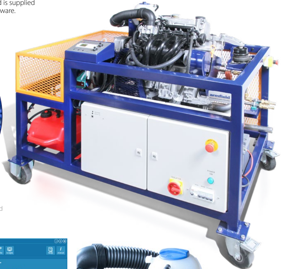
CM11-MKII Integrated eddy current dynamometer to vary engine load
