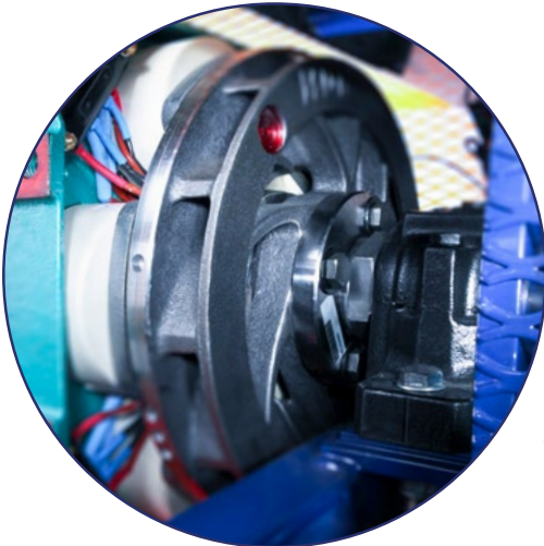
CM11-MKII Integrated eddy current dynamometer to vary engine load
