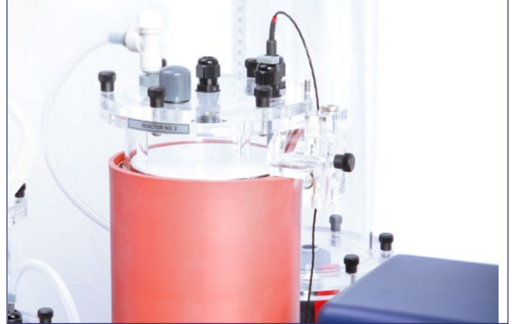
W8 insulated jacket around the reactor
