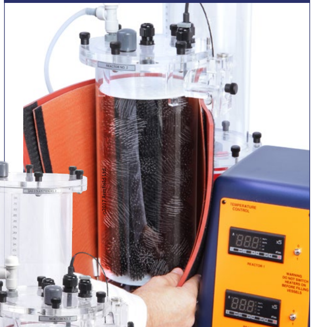
W8 reactor detail showing Bio-balls
