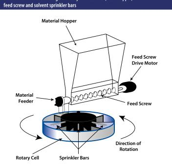
Detail of UOP4Mkll showing the rotary extractor cell, feed hopper,
