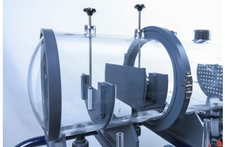
Bucket & Weir design, supplied as standard – Features adjustable bucket and weir height
