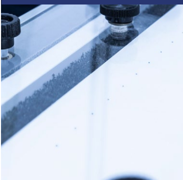
Flow straightener and dye injection system
