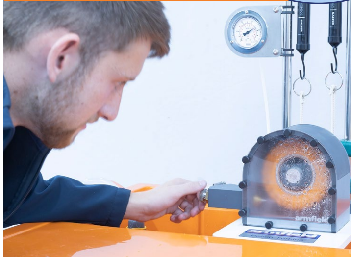
Pelton Turbine brake being operated
