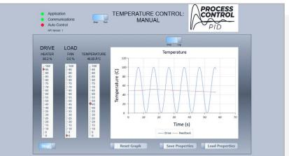
▶ On/Off Control allows students to explore controlling each system with a simple on off algorithm, to see the oscillations this produces and to explore the effects of hysteresis.
