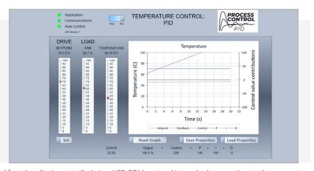
The MATLAB software is supplied with the unit. The Control functionality is controlled via a USB COM port or Networked connection to the computer. We have provided a library of functions to allow the various aspects of the Control Hardware to be investigated and controlled.
