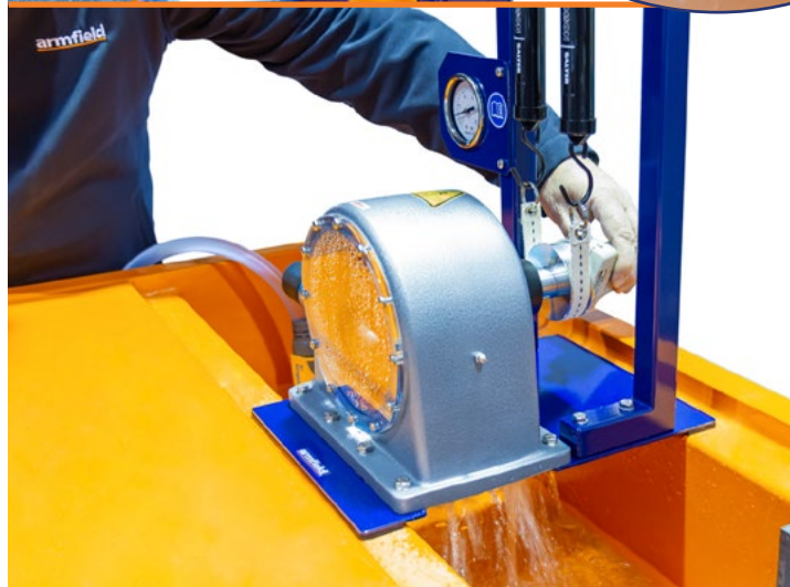
Pelton Turbine brake being operated
