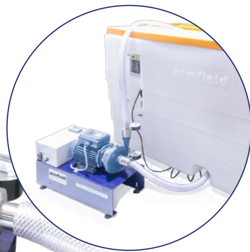
F1-27 Centrifugal pump attached to F1-10 bench
