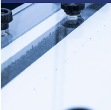
Flow straightener and dye injection system
