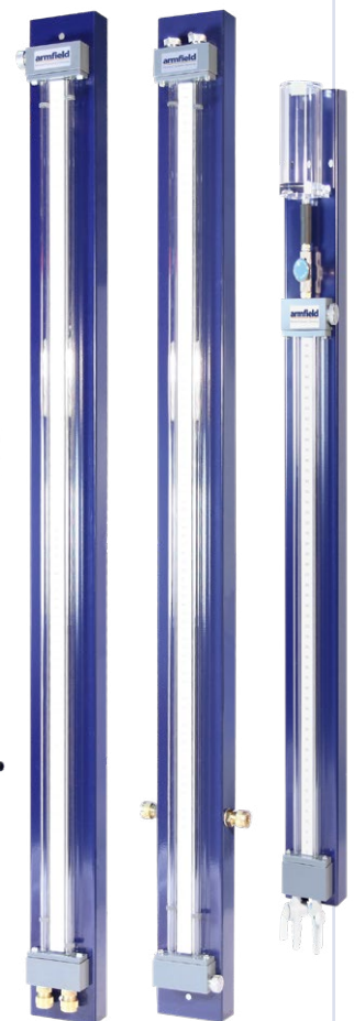
H12-1 to H12-5 Manometers including water, pressurised, kerosene over water
