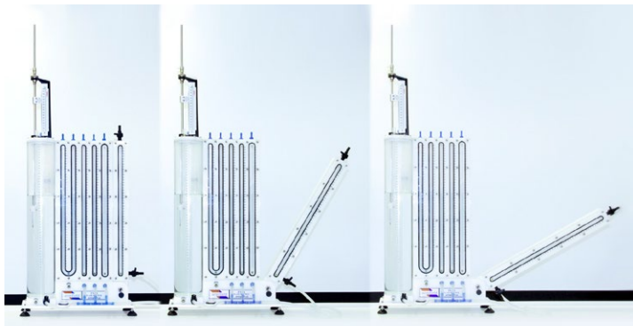
F1-29: Different inclination angles in the inclined manometer
