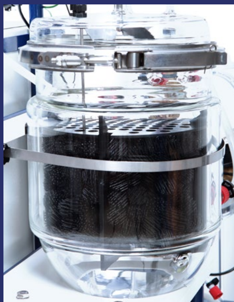
Tank reactor showing detail of bio-balls and supports, configured as PBR (packed bed reactor)
