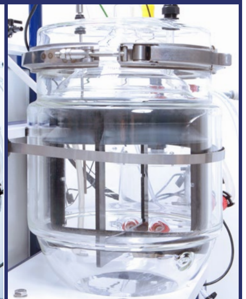
Tank reactor showing detail of baffles, deflector and lid configured as UASB (upflow anaerobic sludge blanket reactor)
