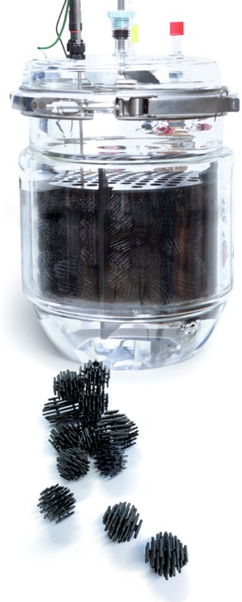
Tank reactor showing detail with bio-balls
