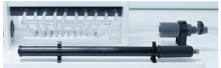
F1-15-MKII: Pump for pressurising the system
