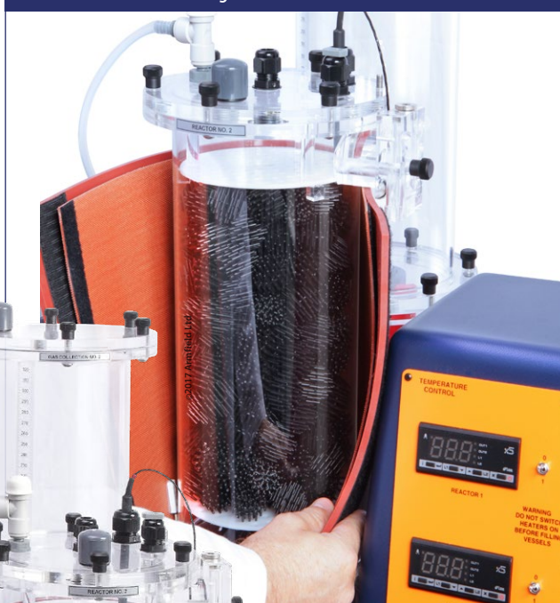
W8 reactor detail showing Bio-balls
