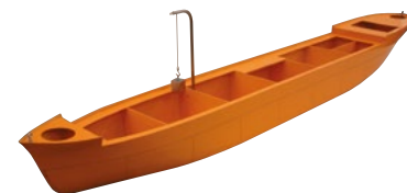
Supplied - 1/70 scale model of a 28000 tonne general cargo vessel
