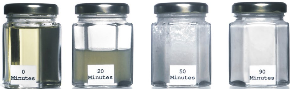
Samples showing the increasing hardness of the oil with process time
