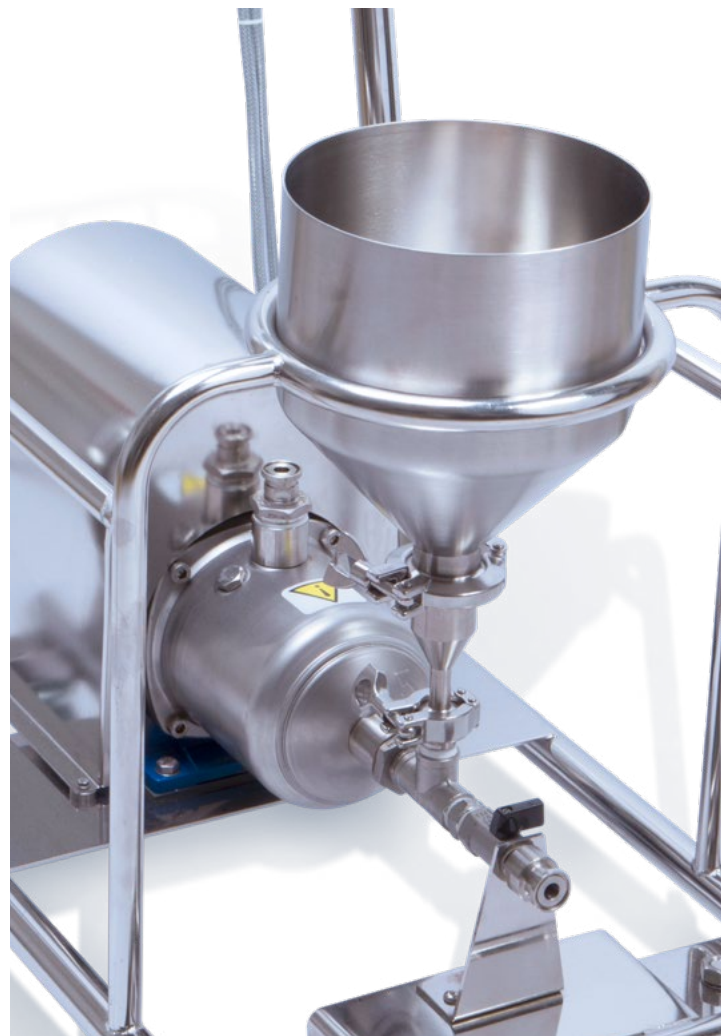
Centrifugal pump and 5L feed vessel
