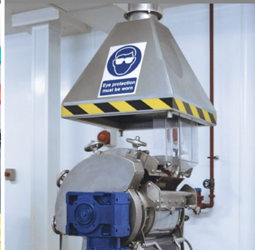
FT32-20 Vapour extraction system
