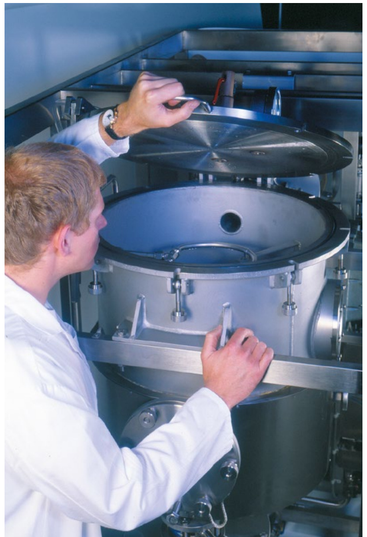
Inspecting the interior of the extractor vessel
