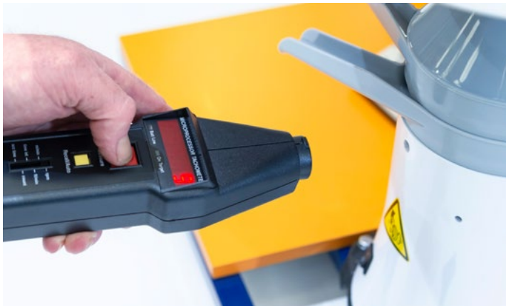
FT15 Optical Tachometer
