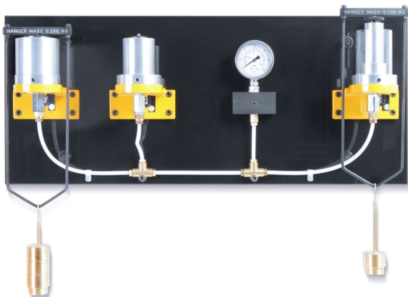
SD-1.27 Simple Hydraulic System
